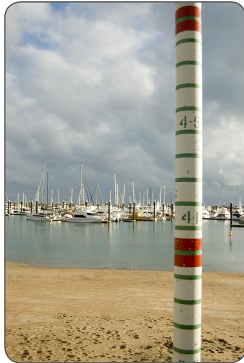
To help show the height of high and low tides, a *tide gauge* indicates the maximum and minimum water levels.
