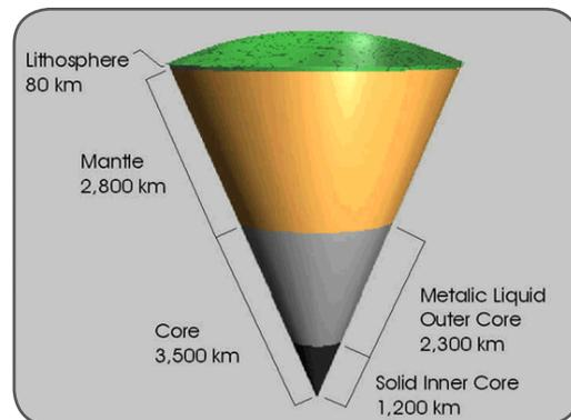
The relative thicknesses of the compositional layers of Earth are shown for comparison. (Image from US Geological Survey)
